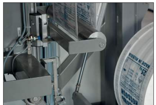
Motorized film roll advance with constant tension
